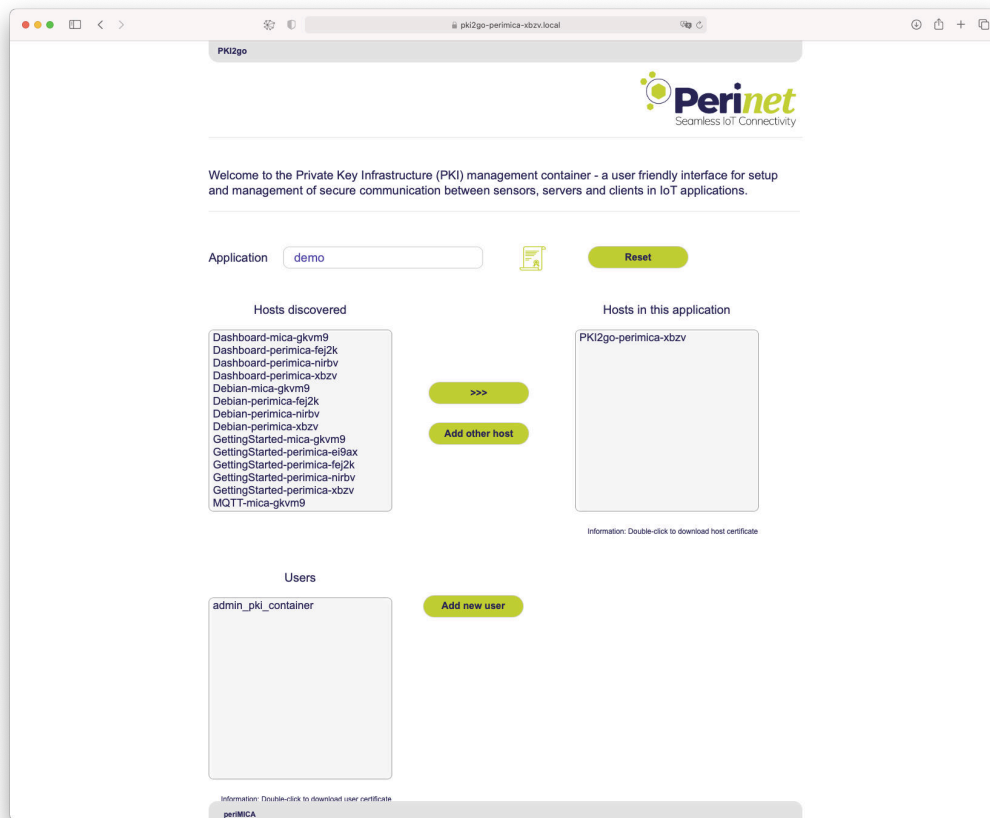
Figure 4: PKI2go container with a demo Root CA setup
